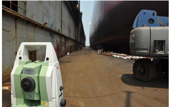
Total Station leica TS30 in action.
