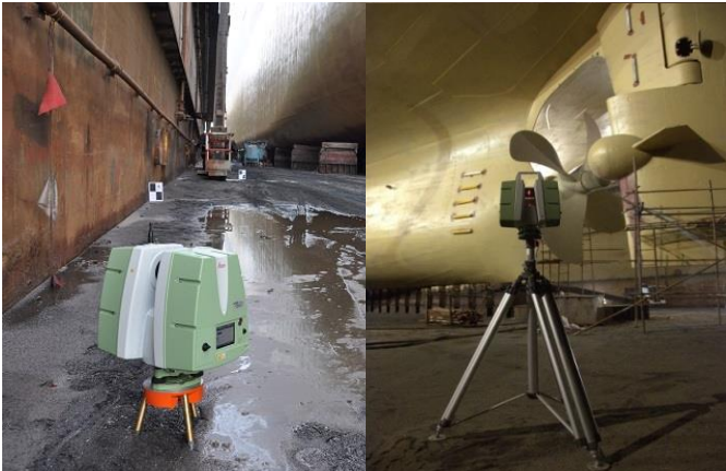
Leica ScanStation P20 in action. Scans were mainly taken during night hours
